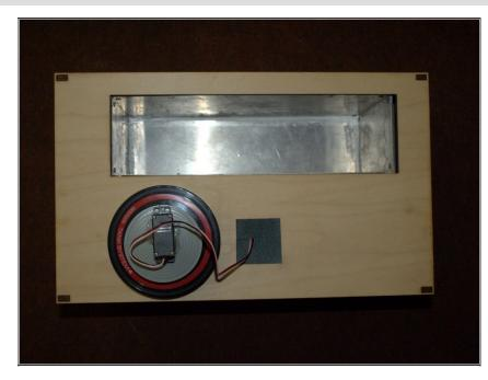
I attached the servomotor to the lid of my developing tank with hot glue, and added a stirrer to the servo shaft using bent wire. To avoid the tank lid being permanently attached to the Photo Lab along with the servo, I added a servo connector to the top, which is wired to the main board's power, ground, and Arduino pin D8 for control.
